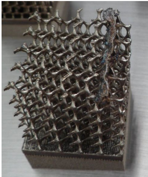
Fig. 5 The margins of the samples a without self-supporting function, b self-supporting function was preserved [14]
